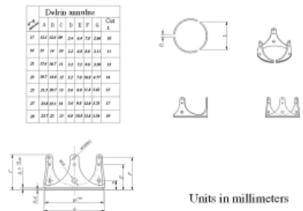
Fig. 2 – Diagram of bioprotheses with its dimensions.
