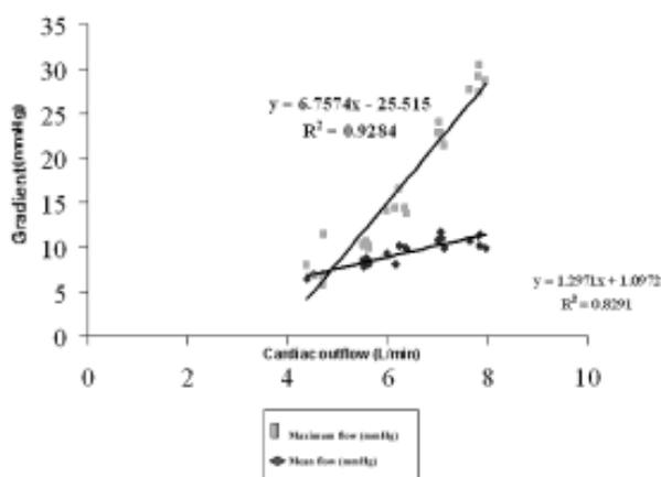
Fig. 3 – Analysis of the transvalvar pressure gradient
